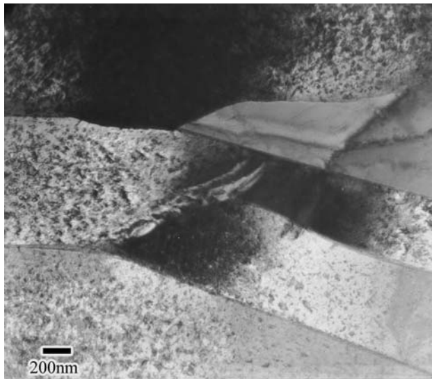
Fig. 3 BF TEM micrograph of a 5N FAB presenting anisotropic grains and a relatively low dislocation density
